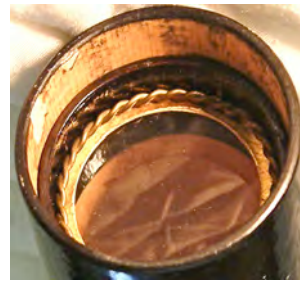
Masakatsu: Eyepiece lenses held by twisted two-wire brass expansion ring
