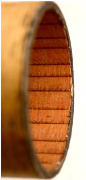
Stave construction of tubes
