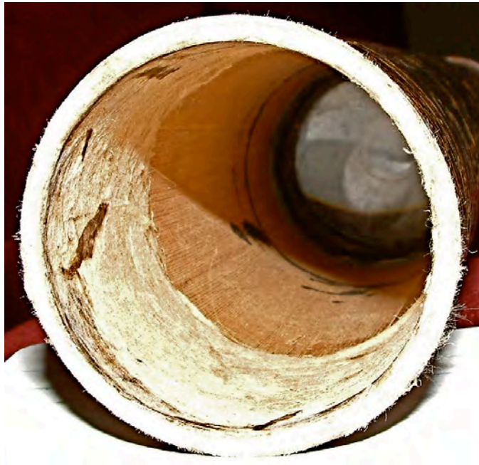
Non-stave construction of tubes
