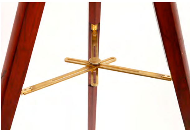
Custom spider: folds down when decoupled
