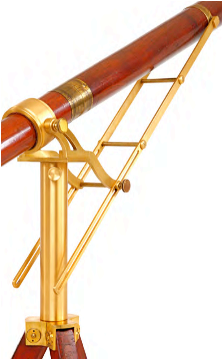
Overall side view. Tension bolt on right slider fixes the viewing altitude Slider can be indexed in degrees for easy reading of the viewing angle.
