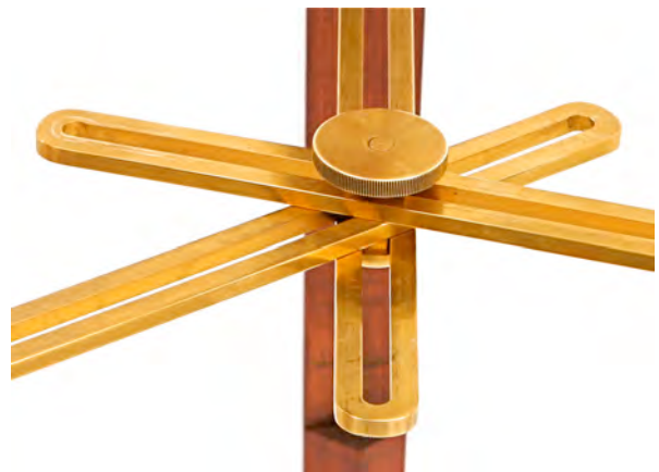
Custom spider with Dollond tightener
