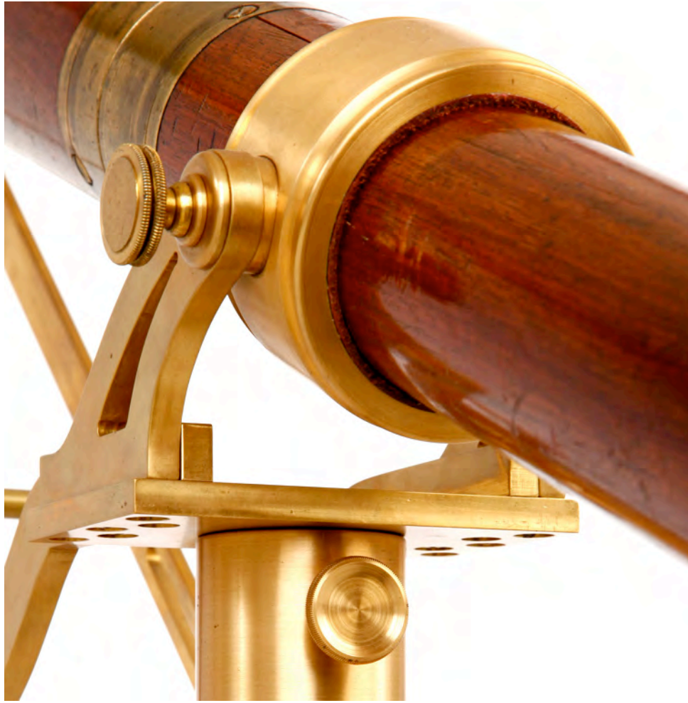
Compression collar supported by hook-type pivot mount.
