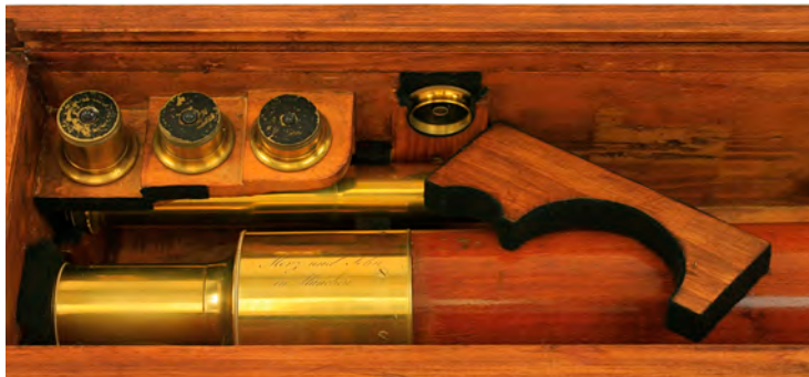
Remounted the solar filter and created new top-half retainer boards that were missing.
